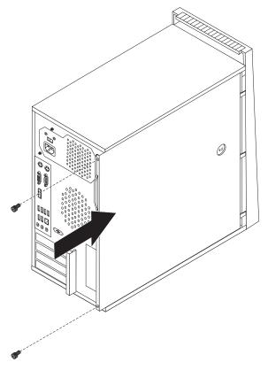
Figure 39. Reinstalling the computer cover
